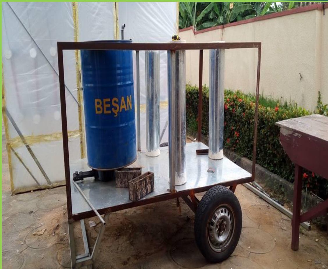
PYROLYSIS MACHINE FOR CONVERTING WASTE PLASTICS TO FUEL
