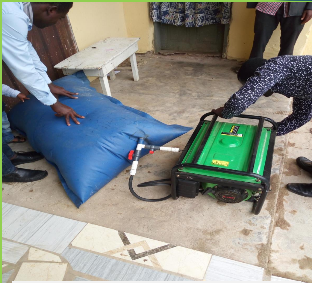
BIOGAS GENERATOR USING BIOGAS ENERGY AS FUEL
